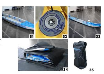
Once you have deflated the kayak, fold the walls over the base so the kayak is ready for a compact, tight fold [34]. Always make sure the skeg/fin slide base is pushed down flat to prevent it from bending and becoming misshapen.
