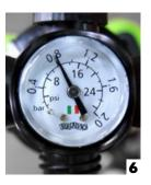
Maximum air pressure for this model is 10 PSI [6]. In extremely warm weather you may wish to let some of the air out when not using to allow for hot air expansion. AVOID over inflation as this will lead to your warranty being declared invalid.
