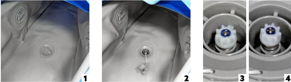
The Bluewave Glider has a recessed valve for each side chamber and the floor [1] to pump air into for inflation. Remove the cap to access the valve [2]. Press and turn the valve counter clockwise so it pops up [3,4]. This will close the valve and hold in air for inflation. Turning the valve clockwise will open the valve for deflation.
