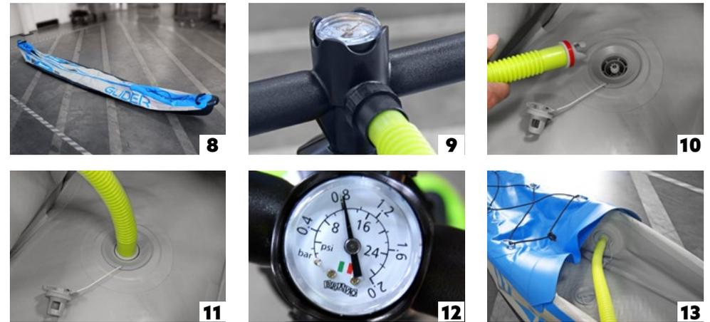
Choose an area large enough to unfold [8] the Glider, ensuring the space is free of hazards which could damage the kayak or cause injury. You can inflate the sides or floor in any order. The working pressure for walls and floor is 10 PSI [12]. The front of the kayak can be identified by the closest sets of D-rings to the splash guards. If the D-rings nearest to the splash guard are positioned lower down to the following D-rings, this is the front of the boat.
